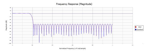
Figure 3.1: A low pass filter design.
