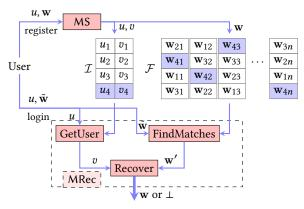
Figure 1: Diagram of multisketch as a part of an authentication service.
