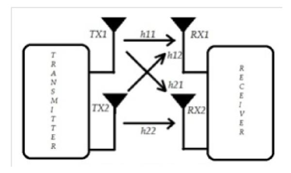
Figure 2: MIMO SYSTEM MODEL.
